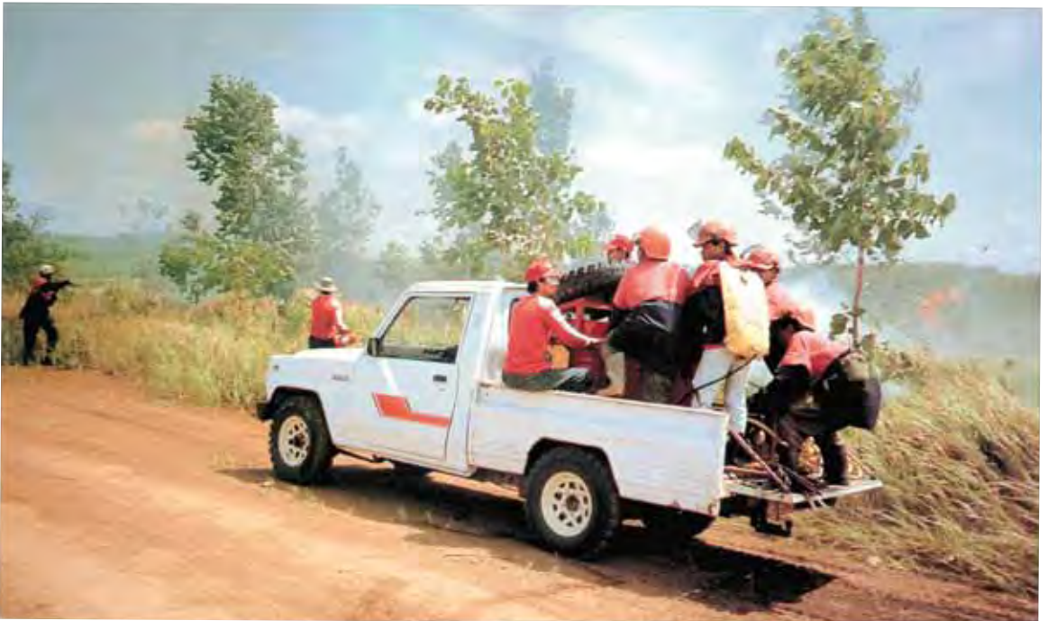
Fire pick-up Attack Unit with crew; equipped with light motorized pump (capacity 80 l/min), knapsacks and fire swatters, Indonesia
